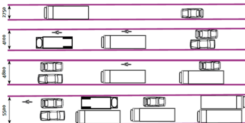
Figure 7: MfS Extract pertaining to carriageway widths
